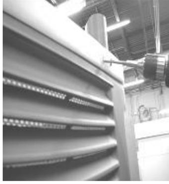
Install (3) 1-1/2" long screws PN 16809 with 5/16" rubber clad washers (3) PN 17626 in the rear corners & in the front right corner.
